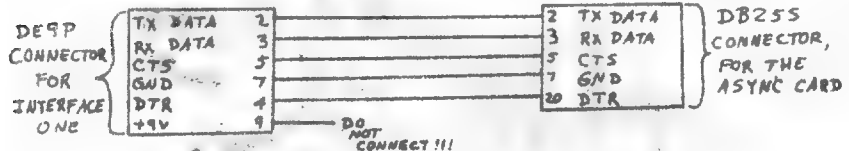
FIGURE 1 CABLING BETWEEN PC AND INTERFACE ONE
